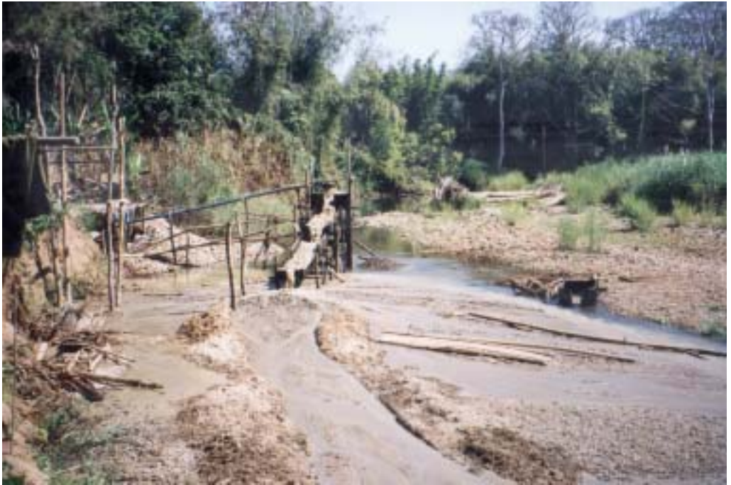
A gravity-fed, multi-level sluice
